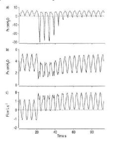
An example of a mask leak at 20 second mark causing swings in the tracheal pressure (top penal), a drop in mask pressure (middle penal), and an upward shift and flattening of air flow. At 50 second mark the device compensated for the leak and increased the mask pressure to baseline levels, normalized the tracheal pressure swings and improved the airflow to round curve. (Adopted from Eur Respir J 2004; 24:649-658)
