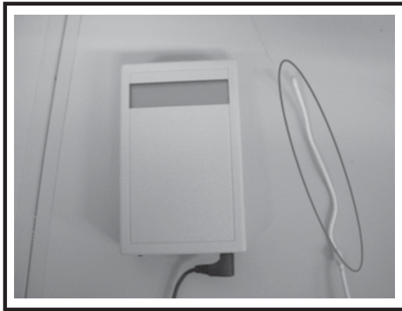
Figure 3: Device to measure rectal core body temperature. Circled part will be inserted into rectum through anus.
